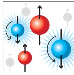
4. When the radio wave pulse is turned off, these protons release energy, emitting a signal.
