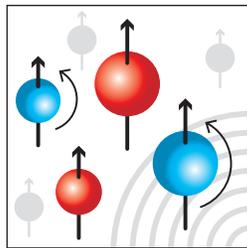
3. Radio frequency (RF) pulses are directed at the body part being imaged, causing certain protons to spin, or resonate, as they absorb the RF energy.
